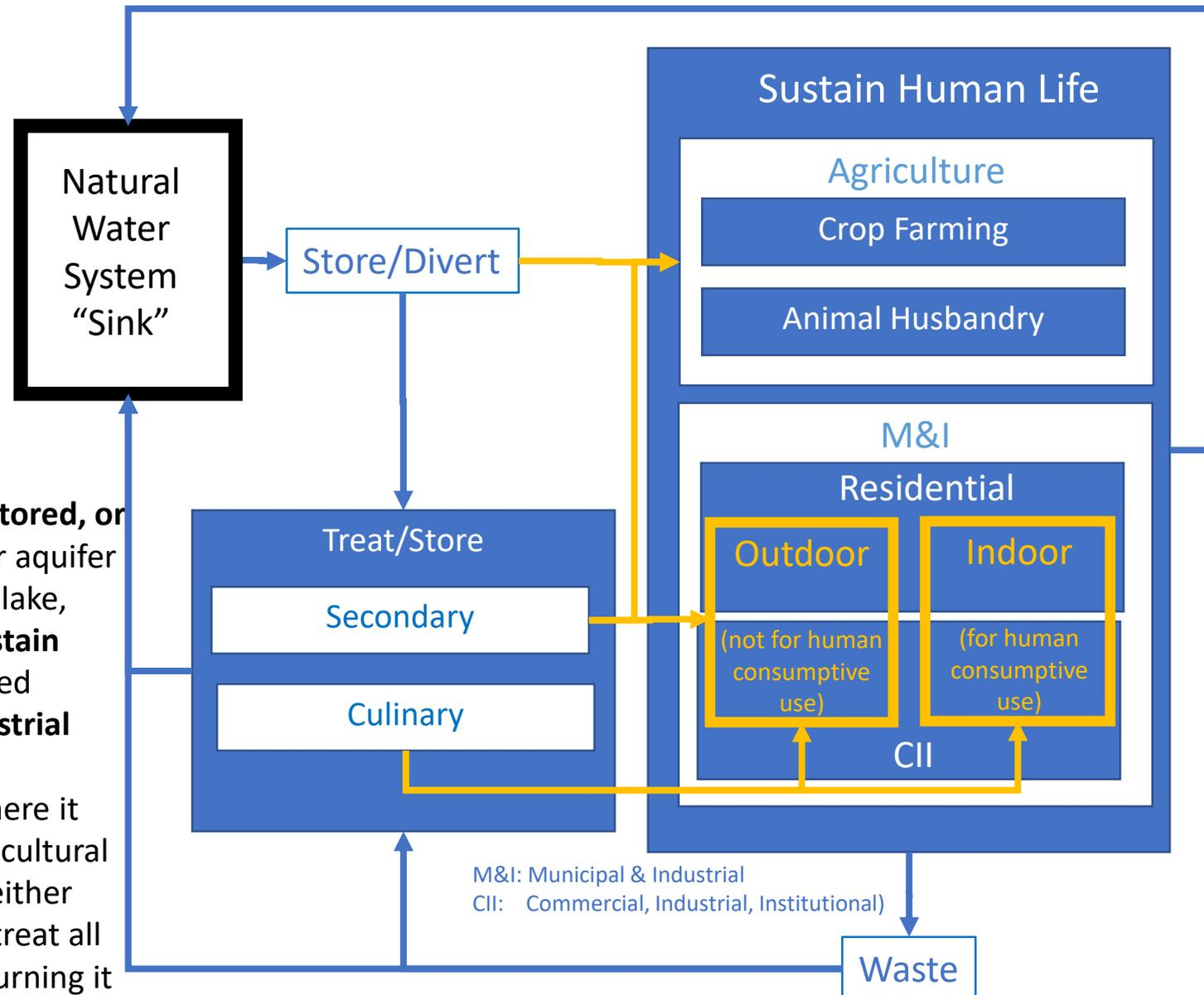
All arrow are “managed flows” using ditches, pipes, and pumps.
