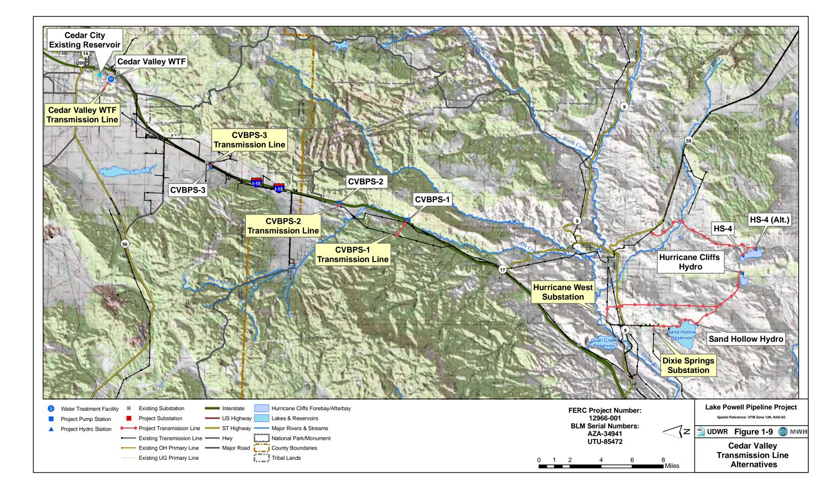
The **Cedar Valley Water Treatment Facility Transmission Line** would begin at an existing substation in Cedar City and run about 1 mile to the water treatment facility site in Iron County, Utah (Figure 1-9).
