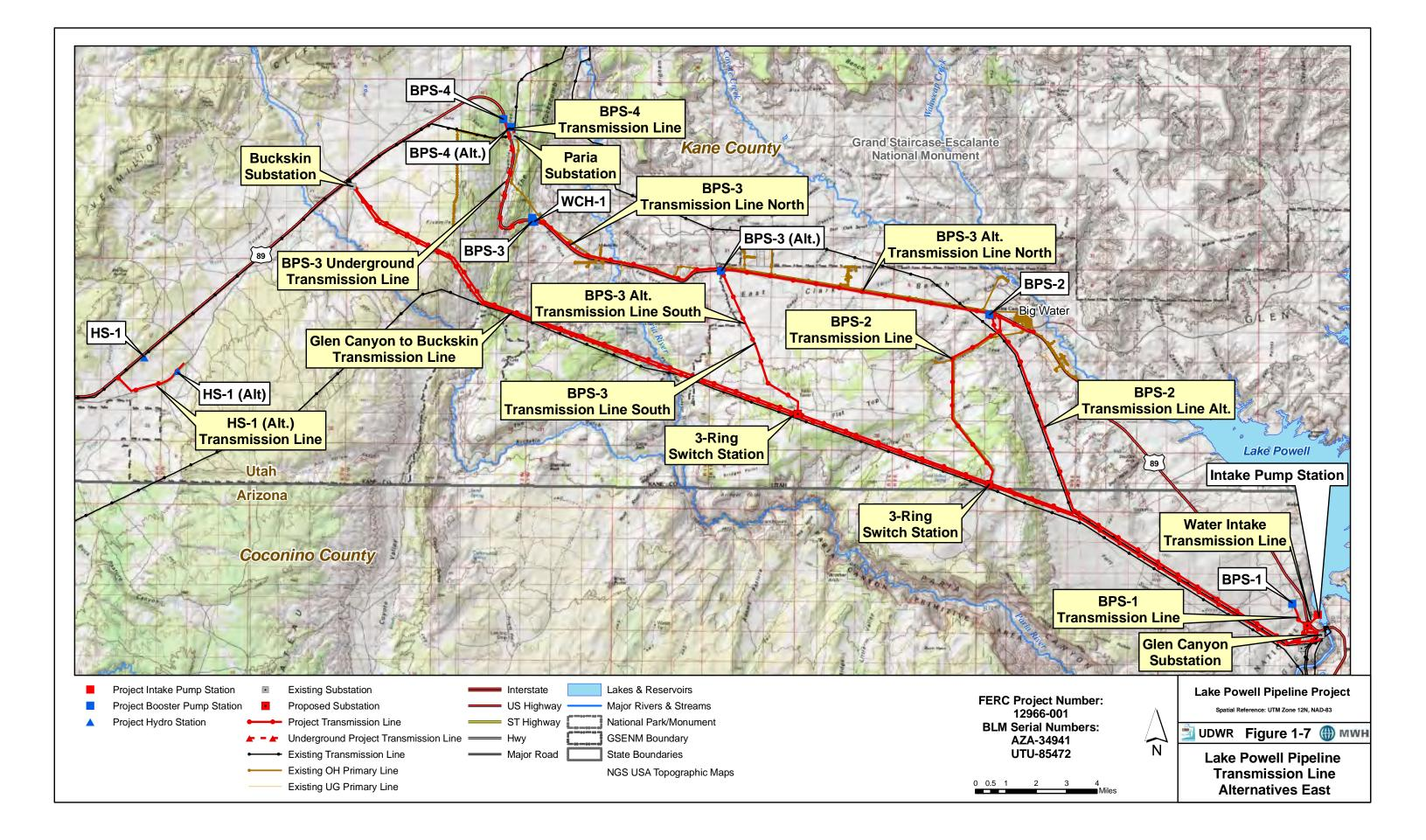
County, Utah. The new transmission line would parallel an existing distribution line that runs northwest, north and then northeast to Big Water. This new 138 kV transmission line alternative would be about 7 miles long across Utah SITLA-administered land, with a 138 kV connection to a new electrical substation on the BPS-2 site (Figure 1-7).
